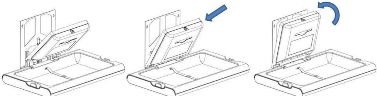
Open the liner dispenser with the special key provided. The four holes for mounting the liner dispenser on the holding structure of the changing station will be visible.
